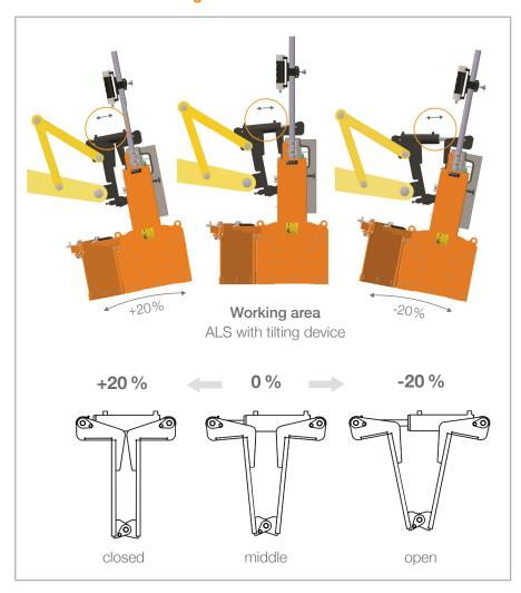
**Variant 2: ALS via tilting cylinder of the loader**
