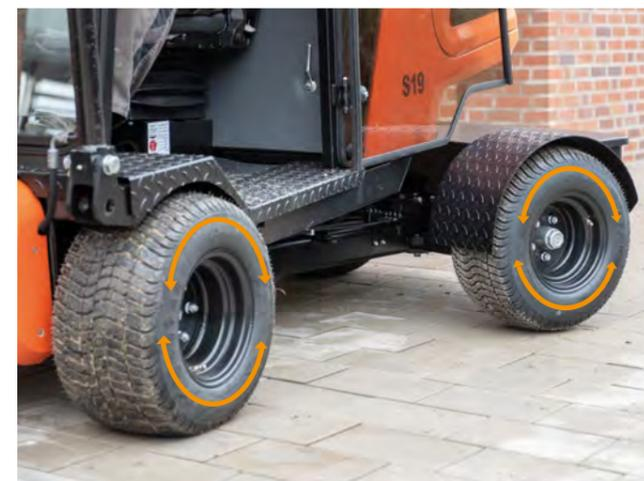
All 4 wheels are driven and braked hydrostatically.
