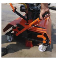
Simple height adjustment to bring brushes into correct position for pushing in the sand.
