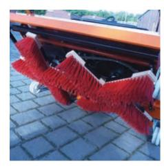
Two rotating brush-crosses generate a Easy to use. Seamless filling of joints without slurry of sand and water allowing joints to be filled completely in one go.
